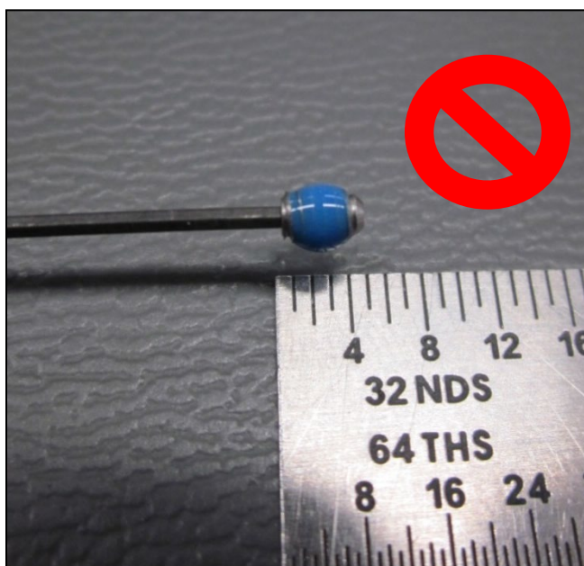
Figure 4: Too much adhesive applied
