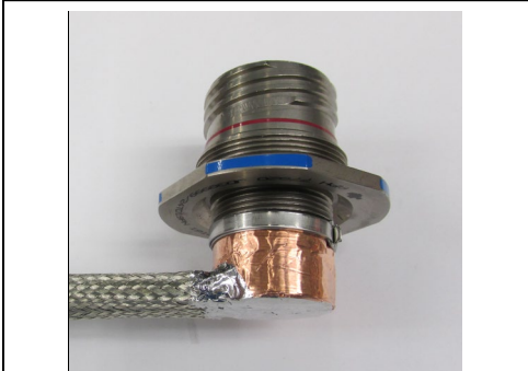
Figure 6 Copper Foil to Threads with Solder and Clamps
