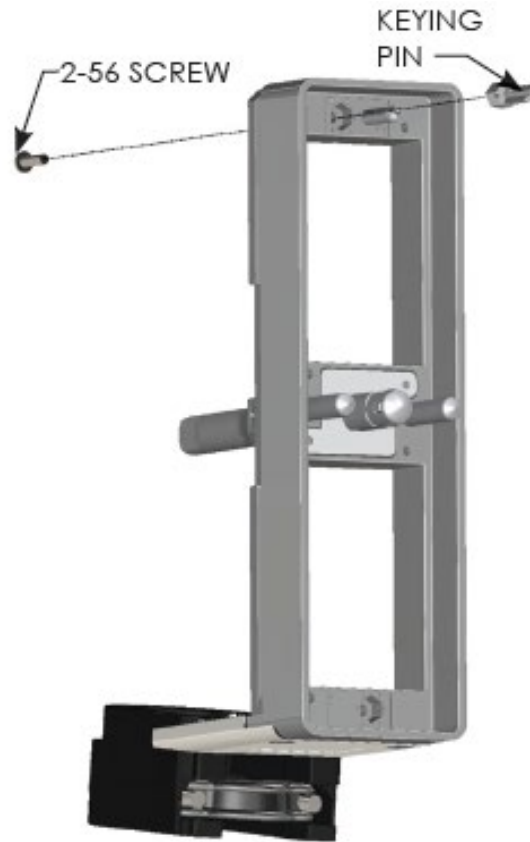
Figure 6: iCon ITA Connector Frame and Keying Pin
