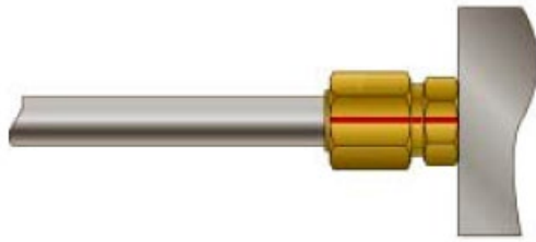
Figure 1: Typical Reference Mark on nut and Tube Body
